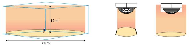
Two adaptable clip-on shielding masks are supplied with the unit. Each can cover half of the sensor lens.
