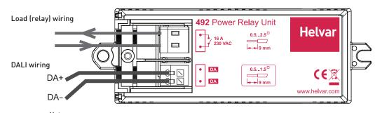
Note: The DA+ and DA- wires can go in either of the DALI connectors.
