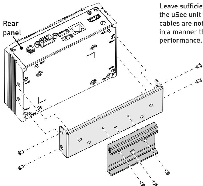
Leave sufficient clearance around the uSee unit to ensure that the cables are not crushed or bent in a manner that may affect their performance.
