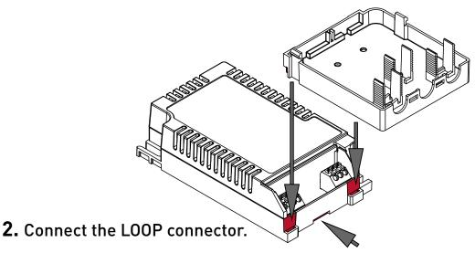
I. Connect the two short wires into LOOP connector.
