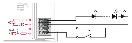
Helvar's innovative Direct Control (patent pending) behaves much like the Switch-Control, but in this case the control can be implemented in a more straightforward way without using the mains voltage. Only a simple retractive (push to make) switch connected into the Iset / LED-Iset terminal and enabling the Direct Control from the Helvar Driver Configurator tool are needed. DALI usage is **not supported** at the same time with Direct Control operation.
